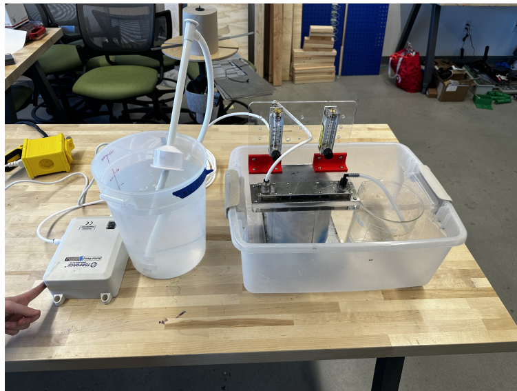
Figure 4.2: Physical assembly of experimental set-up with constant flow pump, fluid reservoir, and wastewater beaker.
