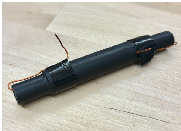
Figure 5.4: Preliminary transducer design prototype with copper electrodes.
